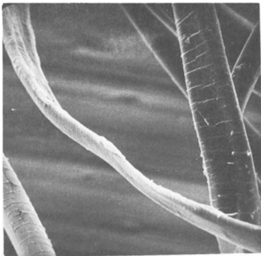
Figure 13 SEM of fibre surface from 24% terylene/polypropylene 543M composites (magnification \times 560 ).
