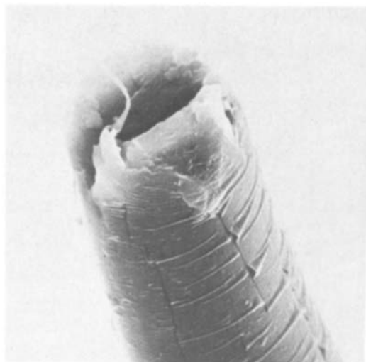
Figure 12 SEM of fracture surface of fibre 24% terylene 11H/polypropylene 8639 composite (magnification \times 2350 ).
